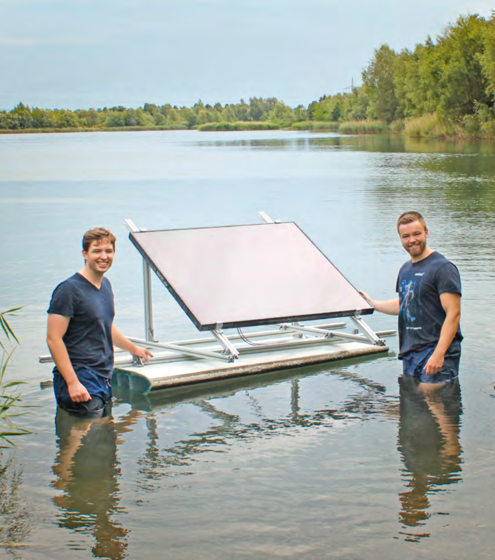
Kevin Strödter (left) and Philipp Johst inspect a solar panel floating on part of an old wind turbine blade
