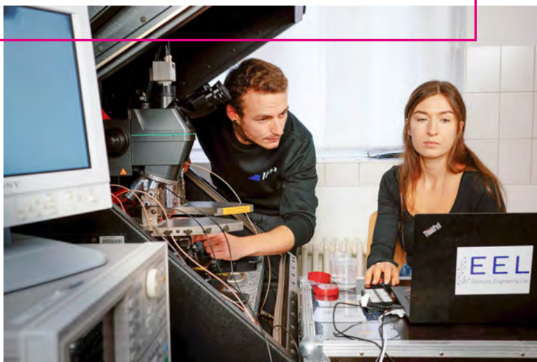
Florian Muschka and Anika Mühl print organic electrochemical transistors
