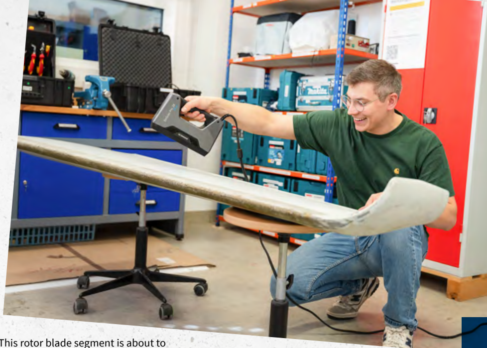
This rotor blade segment is about to become a table. Dimitrij Seibert starts by scanning the piece with a 3D scanner to digitally plan the next steps
