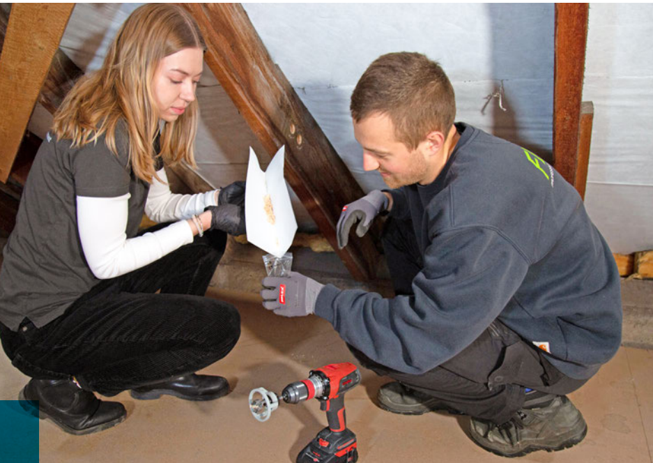
Luisa Sander and Henri von Mulert collect wood samples from a roof rafter for subsequent contaminant analysis
