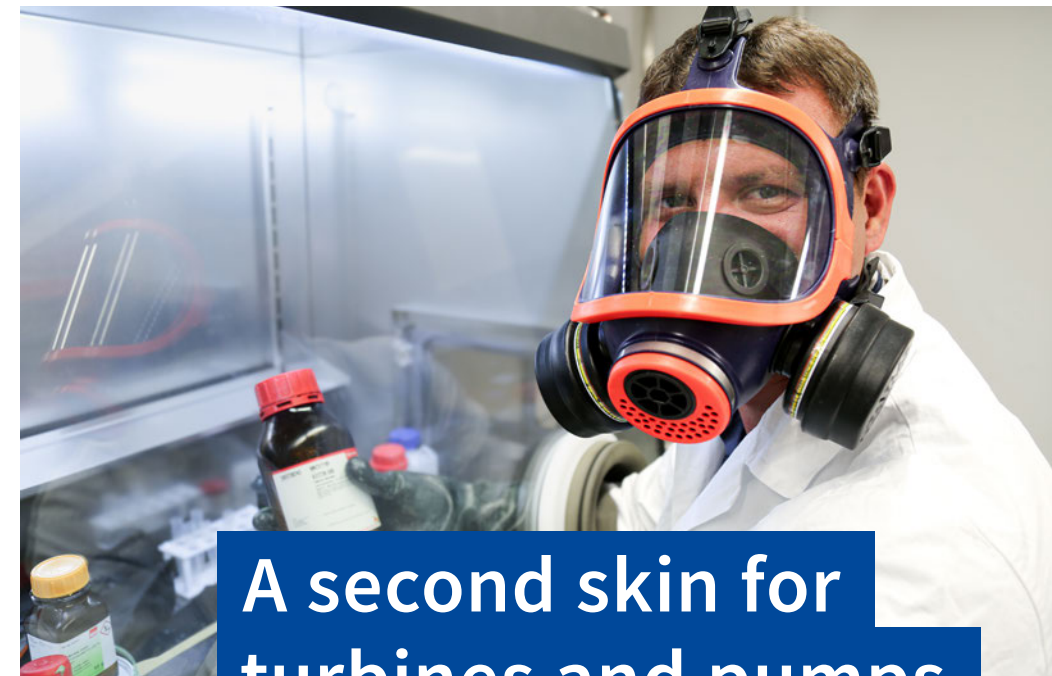
Dr Dmytro Rassokhin mixes nanoparticles into a polymer compound in a glovebox
