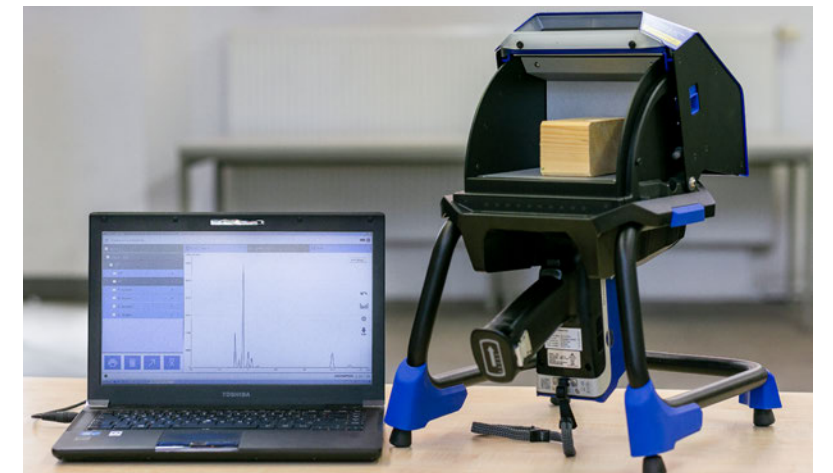
The researchers used a mobile X-ray fluorescence device to analyse a sample treated with wood preservatives
