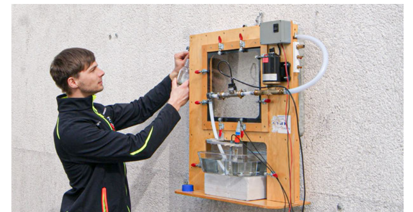
This rainfall simulator recreates rainwater running down a façade. Robin Berg collects a water sample to analyse which biocides are leaching from the material
