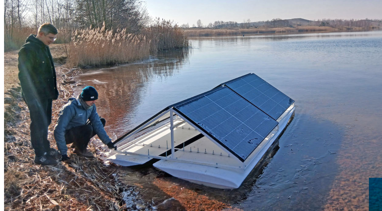
Dimitrij Seibert (left) and Jan Bürgener test a floating photovoltaic system on a lake in Leipzig, mounted on old wind turbine blades
