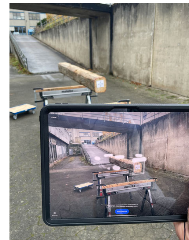
The researchers have also developed a piece of technology that uses 3D scanning to digitally estimate how much usable timber is available
